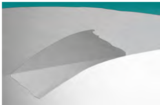
Tohoku subduction zone: CAD model and tetrahedral mesh (C. Pelties)
