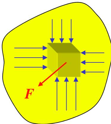
$$\sigma_{ij}(\vec{r}, t) = \underbrace{B}_{\text{Bulk modulus}} \vec{\nabla} \cdot \vec{u} \delta_{ij} + \underbrace{S}_{\text{Shear modulus}} \left( \frac{\partial u_i}{\partial r_j} + \frac{\partial u_j}{\partial r_i} - \frac{2}{3} \vec{\nabla} \cdot \vec{u} \delta_{ij} \right)$$
