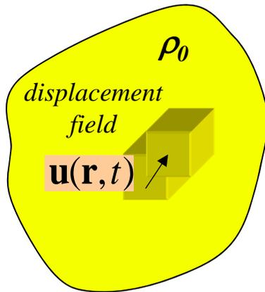
$$\rho_0 \frac{\partial^2 \mathbf{u}(\mathbf{r}, t)}{\partial t^2} = \underbrace{\vec{\nabla} \cdot \vec{\boldsymbol{\sigma}}(\mathbf{r}, t)}_{\text{Internal Force}} + \underbrace{\mathbf{F}(\mathbf{r}, t)}_{\text{External Volume force}}$$
