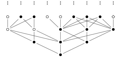
Note that on level 2, the  $\circ$  nodes and the  $\bullet$  nodes have different predecessors, so cannot have any common successor. This introduces branching.
