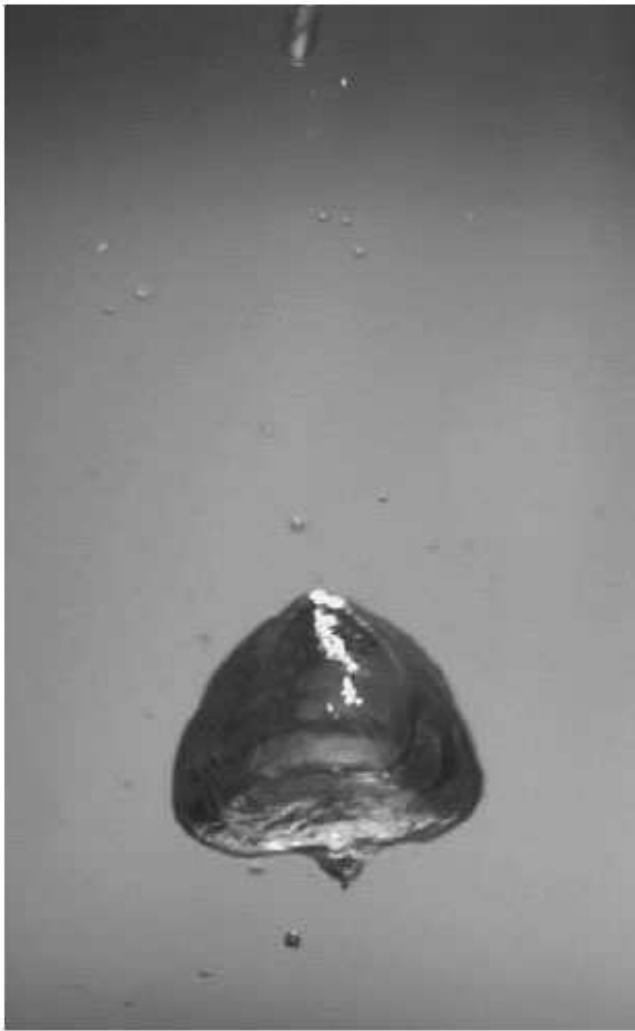
Figure 5: inverted heart shape in experiment by Akers & Belmonte '06: air bubble rising in a polymeric fluid
