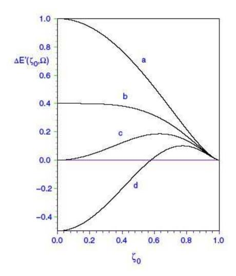
Plot  $\Delta E'(r_0, \Omega)$  as function of  $\zeta_0$  for various fixed  $\Omega$  [9], where  $\zeta_0 = r_0/R_0$  is scaled displacement from center
