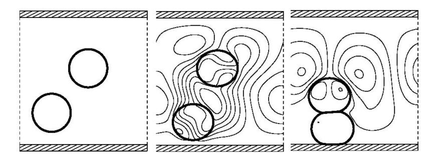
The motion of two oblate drops in a quiescent flow. The drops align with the electric field and attract each other. The drops are also attracted to the wall
