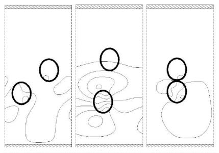
Drop distribution and streamlines for the interaction between two prolate drops.  $S^{-1} = 0.01$ , R=0.1; initial distance between the drops centroids  $r_0=3.5$  times the radius
