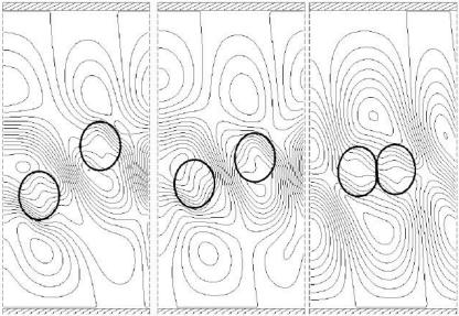
Drop distribution and streamlines for the interaction between two prolate drops.  $S^{-1} = 0.01$ , R=1.0; initial distance between the drops centroids  $r_0=3.5$  times the radius
