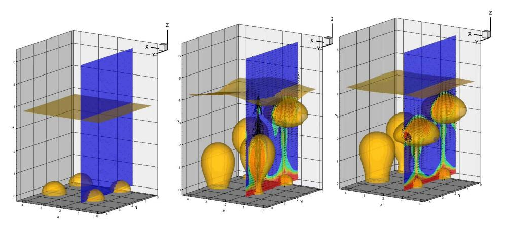
Water at 1atm, Tsat=373.15K; liquid/vapor density ratio=1605; viscosity ratio=23; thermal conductivity ratio=27; specific heat ratio=1; domain size: 10.5x10.5x15.75 mm; Wall superheat: 18K 40x40x60 grid resolution
