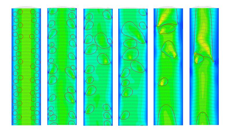
A simulation of a coalescence induced regime transition in a small three-dimensional system
