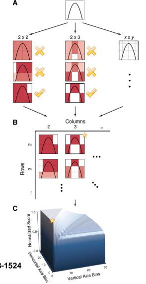
Computing MIC For each pair (X, Y), the MIC algorithm finds the x-byy grid with the highest induced mutual information.
