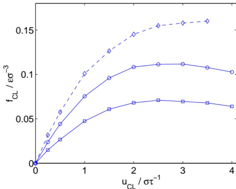
For simple fluids, the nonlinearity sets in at extremely large contact line speed ( $1\sigma/\tau \approx 158\text{m/s}$ ).
