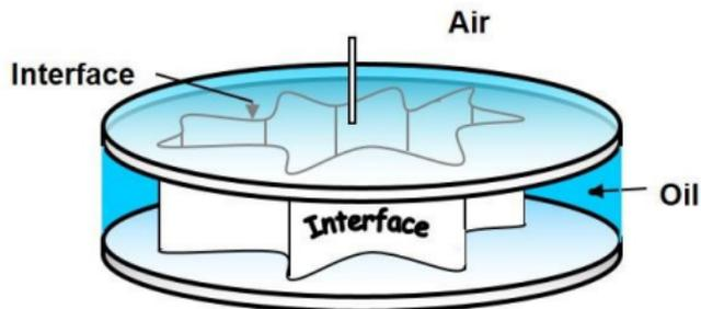
**Experiment:** two parallel, closely spaced plates sandwich a viscous fluid; another less viscous fluid is injected into the system; the interface experiences **Saffman-Taylor instability**.
