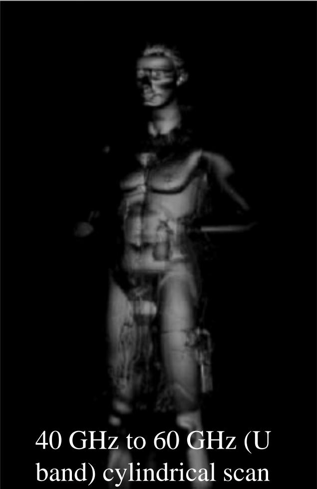
40 GHz to 60 GHz (U band) cylindrical scan
